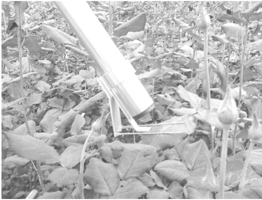
Fig. 1 Fluorescence measuring apparatus with clamped leaf.
